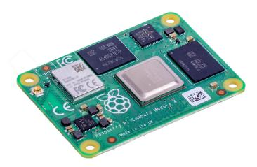
Raspberry Pi Compute Module 4 harnesses the compute power of the popular Raspberry Pi 4 Model B, bringing it to a smaller form factor suitable for integration into products.
